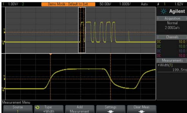
Figure 2: The "Digital Burst with Infrequent Glitch" signal is used to teach students how to trigger the scope on complex digital signals and how to perform more advanced measurements.
